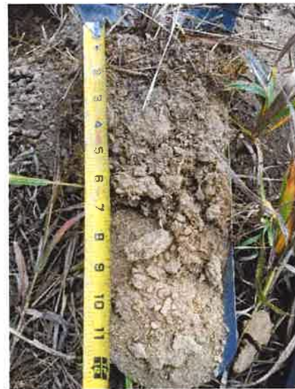
Photo 24 – No hydric soil indicators were observed, and saturation and a water table were not encountered within 24 inches.
