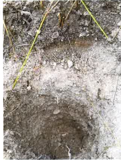
Photo 30 – No hydric soil indicators were observed Community 13; however, the soil pit could not be extended beyond 12 inches.
