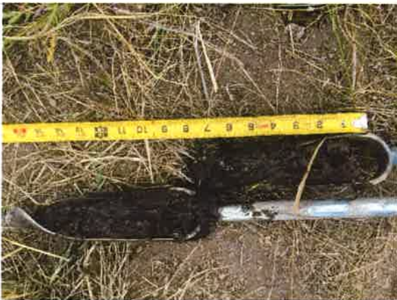
Photo 3 – Soil core from Community 2 exhibited hydrogen sulfide odor and satisfied criteria of thick dark surface
