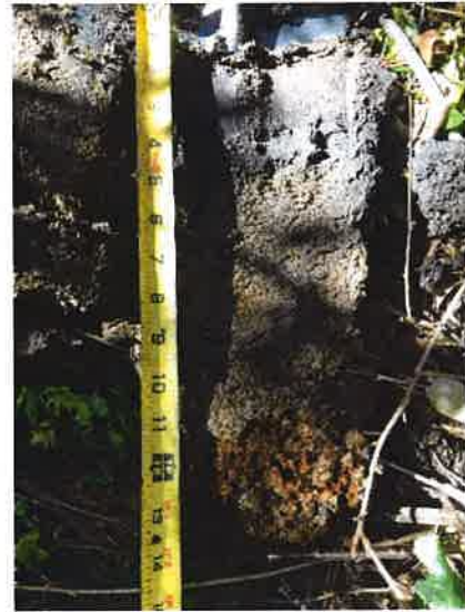
Photo 22 – A hydrogen sulfide odor and sandy mucky mineral soils were observed within Community 9.
