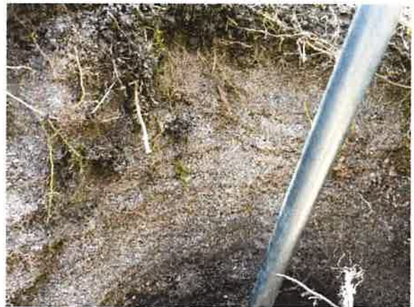
Photo 20 – No hydric soil indicators were observed within Community 8B, the natural sand levee of the Site's stream valley.
